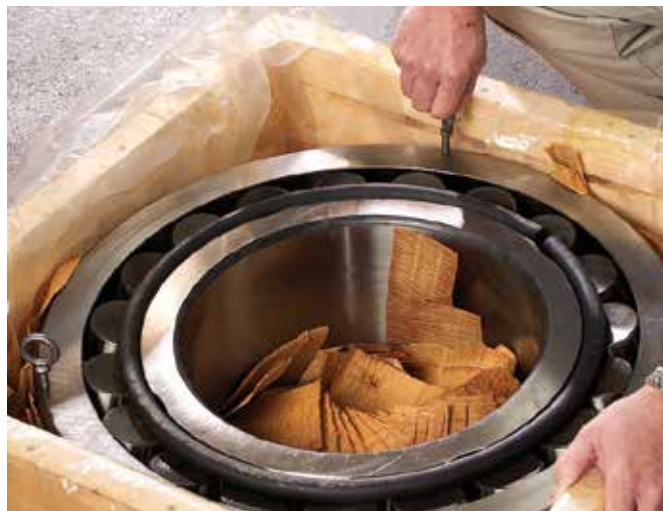
Fig. 2. Eyebolts can be inserted into lifting holes.
