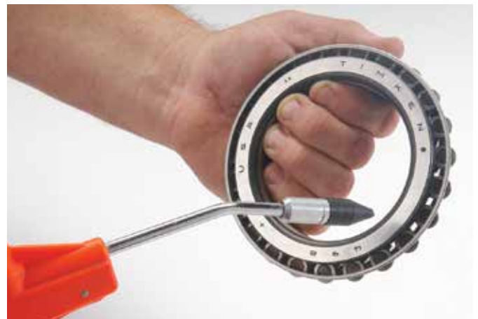
Fig. 19. Drying a bearing.
